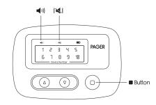
To select another notification mode, press and release the UP Button or DOWN Button on the front of the Pager. The next notification light include will start blinking. Continue to press and release the Up or Down buttons until the desired notification light is selected. Once you've landed on your desired notification light, press and release the Button, you will hear a 1 second beep and/or feel a 1 second vibration. This means the current notification mode is recorded to the Pager.
